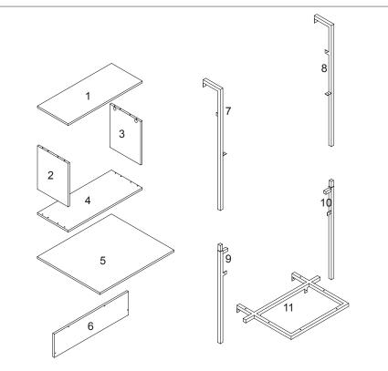
Attach piece 2 & 3 to piece 4 using wooden dowels (G), screws (C).
